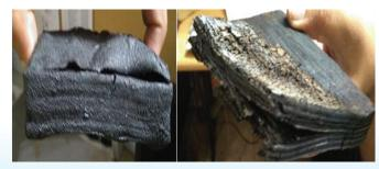
Coated v/s bare wood specimen at 400°C
