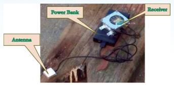
NavIC Messaging and Positioning Receiver Setup with power bank and Antenna
