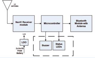
Block Diagram NavlC Messaging and Positioning Receiver
