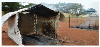
Fig. 1 Model huts made of thatched coconut leaves set to fire. (Left)-Hut without CASPOL coating gutted completely in fire within a few seconds whereas CASPOL coated hut remained intact even in fire.
