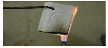
Fig. 2 Images of commercial polyurethane foams set to fire. (Left)-foam without CASPOL impregnation burned completely in fire within a few seconds whereas CASPOL impregnated foam (right) remained intact even in fire
