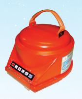
Space Applications Centre (ISRO) has developed the Distress Alert Transmitter-Second Generation(DAT-SG) which is a UHF transmitter based on NavIC receiver module. This NavIC receiver module supports position determination
