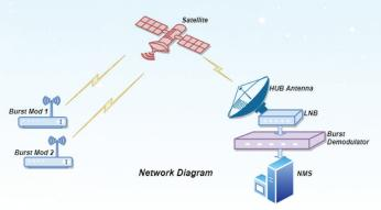
Typical Diagram of SATCOM link with Burst Demodulator
